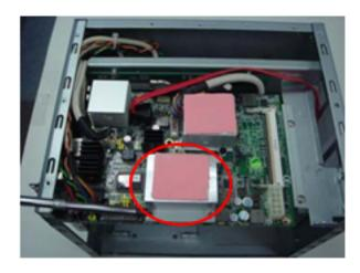
Step 7 Close the top and side covers back to the chassis, and fasten all screws.
